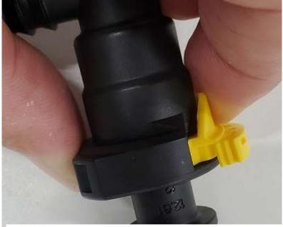
Tab Unlocked, Button pressed to release
