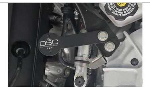
Use the supplied screws and attach J&L Separator to the bracket as shown below.
