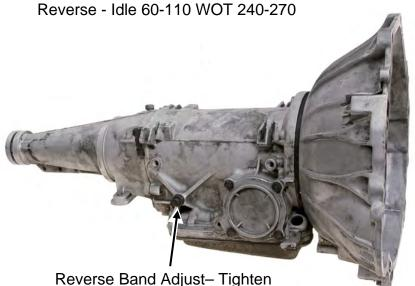
Reverse Band Adjust— Lighten snug with a short wrench and back off 3 turns.
