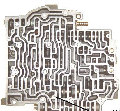
TransGo 00 00 **CUSTOMIZING:** If the 2nd piston casting code ends with 093 or 95-1 0 drill holes A & C .093 to .110 0 0 0 . AUX O 0 00 0 0 000 If the Trans **HAS** auxiliary valve body, plug this hole
