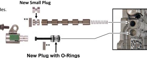
Install **both** o-rings into grooves on **each end** of new plug as shown and lubricate them generously. Using the supplied bolt as a handle, wiggle the new plug as each o-ring **enters a partition**. Do not force the plug! Wiggle and push slightly as you go until the new plug bottoms in the bore. Remove the bolt and install the retain as shown into the groove in the middle of the plug.
