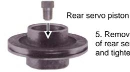
5. Remove check valve and spring from bottom of rear servo piston. Place furnished plug in hole and tighten 4 to 5 turns.
