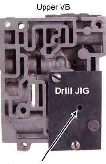
1/16 to 5/32 Drill here through casting.
