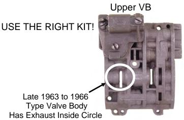
1. Remove valves from upper VB, install drill jig as shown. With any drill from 1/16 to 5/32, drill VB using jig as guide. Clean casting before reassembly.
