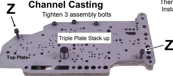
Install with new longer bolts furnished. Two new hex head bolts are for the filter.
