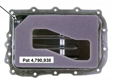
The normal valve body filter **MUST** be used with the dirt diaper. The dirt diaper is **NOT** a replacement for the VB filter.
