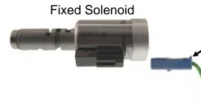
**Grind bump off** on all linear Solenoid Connectors
