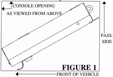
Figure 1 shows the outline of the console opening and proper orientation for placement.
