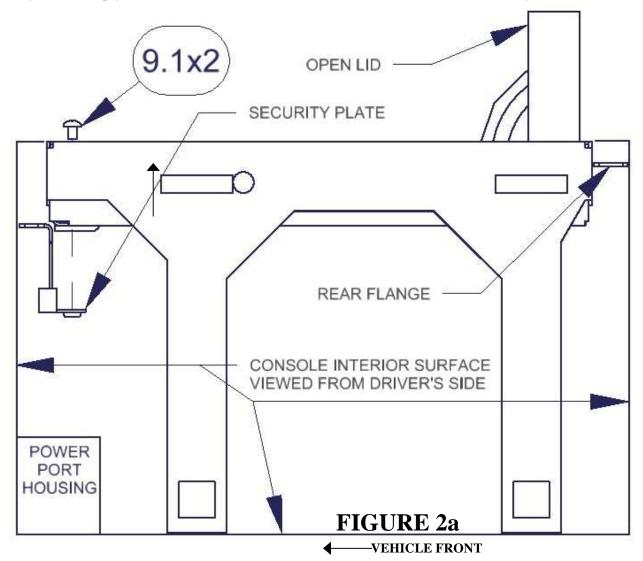
9. Align the holes in the Security Plate with those in the Insert (See Figures 2a, 2b), insert and tighten the 2) #9.1 screws.
