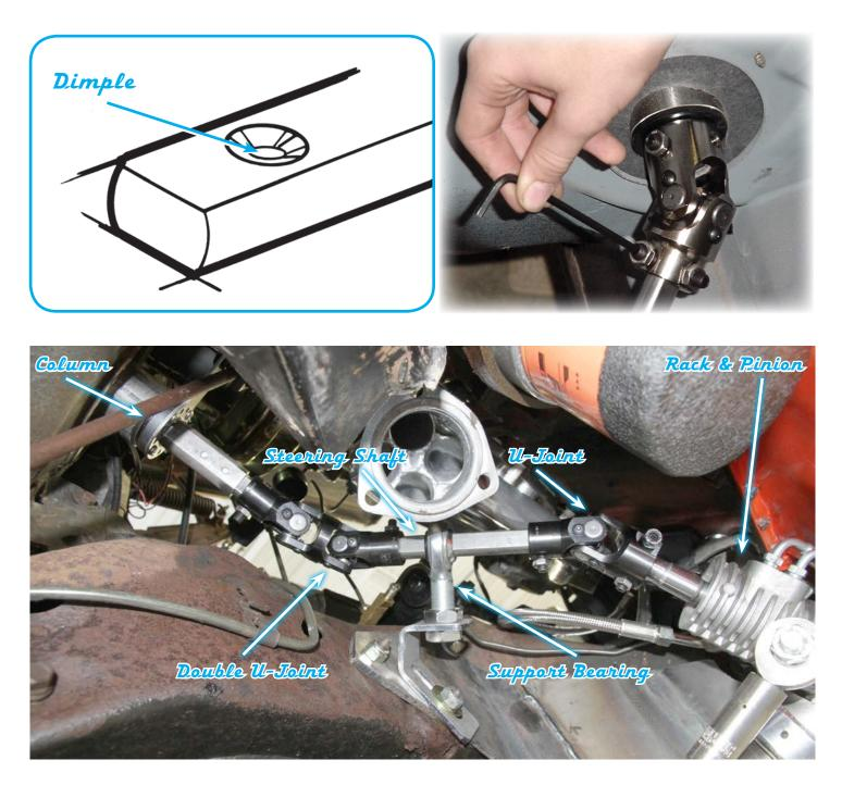
1) Using a 3/4" wooden dowel rod, mock up the steering shaft to obtain the correct shaft lengths and u-joint angle.
