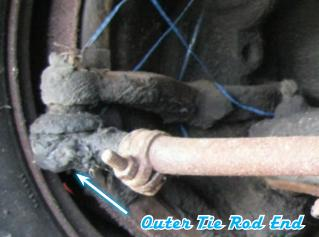
6) Remove the bolts that hold the idler arm bracket to the frame, the outer tie rod ends from the spindle arms, then remove the steering linkage from the car.
