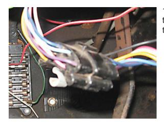
1) Disconnect the wiring at the steering column under the dash.
