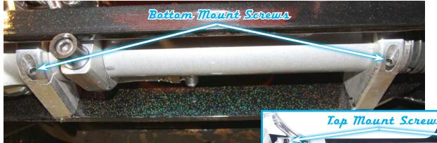
2) The Rack and Travel Bar Assembly comes mounted to the cradle, but can be adjusted to achieve different pinion angles by loosening the screws in the mounts and rotating the rack. Once it is positioned at the desired angle re-tighten all fasteners and make sure to tighten the set screw in the middle of the mount.
