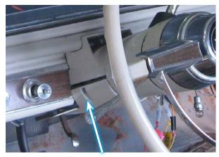
2) Remove the screws and dash bezel
