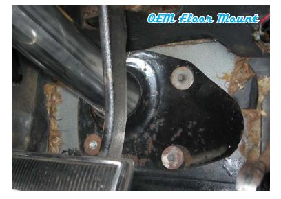
1) Install the original column mounting bracket onto the new Flaming River Tilt Column.
