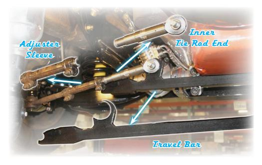
3) Install the OEM tie rod end and the adjuster sleeve onto the new inner end assembly. Note: If using the original parts, some adjustment of the tie rod assembly may be required when connecting to the spindle arm and the travel bar.
