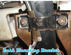
3) Remove the bolts retaining the column dash mounting bracket and floor mounting plate.
