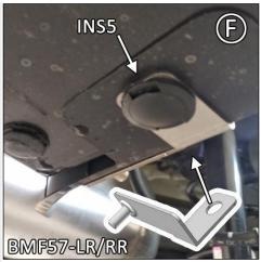
**FIGURE H** Install 1SS and SMWASH into mounting points 1-3. Fasten SSLNUT and SMWASH into point 4, tightening just until mud flap is level with bumper. Do not overtighten.
