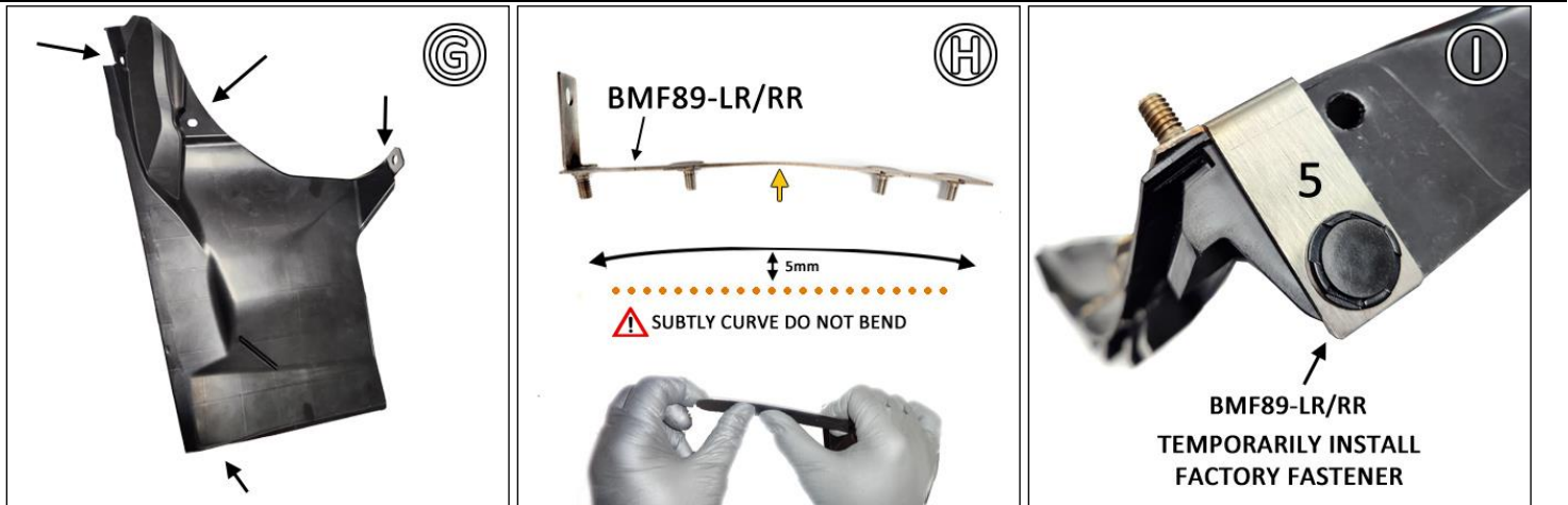
FIGURE J/K Align top-end tab 1 of BMF89-LR/RR to edge of liner before securing UNUT over it. Fasten UNUT over tabs 2 & 3.
