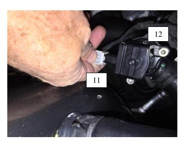
13. Install your new Turbosmart BOV. Align the mounting holes with the flange. As can be seen in the image, the plumb back port of the blow off valve should be facing the plumb back pipe. Holes are not evenly spaced. The BOV will only be installed in one way. Do not force the BOV in, damage will result.
