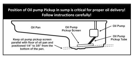
**NOTE**: It is strongly recommended that you tack-weld the oil pump pickup tube to the pump housing, this will provide a solid connection between the pump and pickup tube to prevent separation during severe use or vibration.
