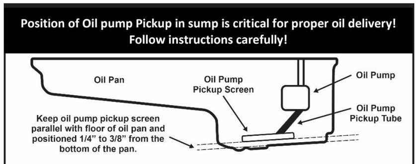
**NOTE:** It is strongly recommended that you tack-weld the oil pump pickup tube to the pump housing, this will provide a solid connection between the pump and pickup tube to prevent separation during severe use or vibration.
