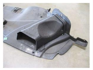
Fig. 11-a: Front brake cooling ducts
