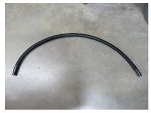
Fig. 9-n: 44" length of the 3/4" coolant hose
