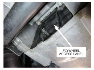
Fig. 3-f: Remove transmission access panel
