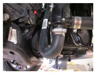
Fig. 9-x: Install coolant hose to electric water pump inlet
