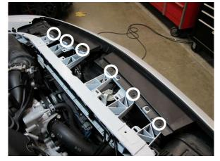
Fig. 2-b: Remove six plastic fasteners
