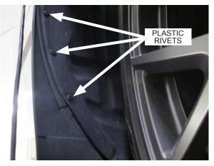
Fig. 11-c: Resecure using provided plastic rivets
