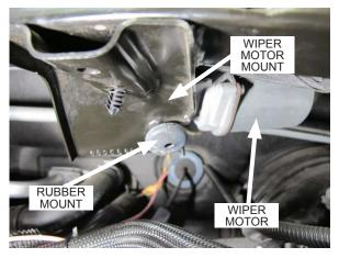
Fig. 1-f: Windshield wiper motor mount
