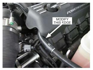
Fig. 11-d: Modify driver side engine cover
