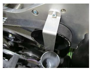
Fig. 6-j: Reinstall pulley guard
