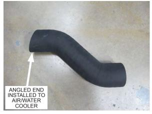
Fig. 7-t: Discharge sleeve 'C'
