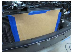
Fig. 7-b: Cover A/C condenser with cardboard
