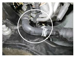
Fig. 5-f: Install 90° end of new coolant reservoir hose to plastic tee
