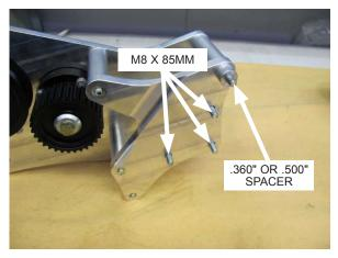
Fig. 6-d: S/C mounting bracket hardware
