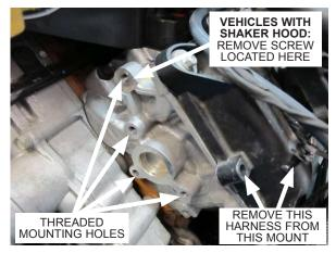
Fig. 6-e: Driver side cylinder head
