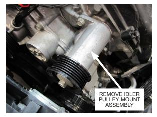
Fig. 2-z: Remove idler pulley mount assembly
