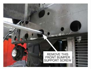
Fig. 9-g: Remove front bumper support screw
