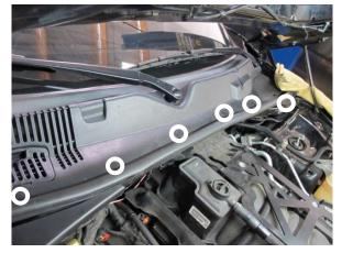
Fig. 1-b: Remove plastic fasteners
