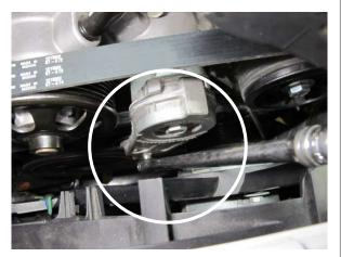
Fig. 2-y: Remove accessory drive belt
