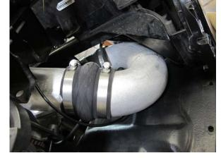
Fig. 7-ac: Loosely install discharge tube 'A' to discharge tube 'B'
