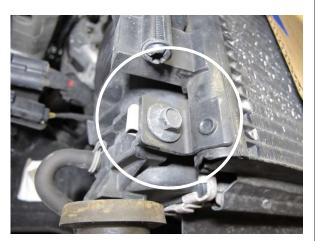
Fig. 7-d: Remove screw
