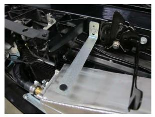
Fig. 10-a: 1.00" width radiator shroud bracket with rubber mount
