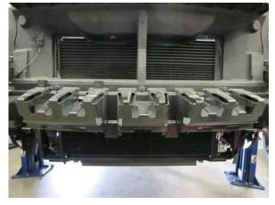
Fig. 2-k: Remove plastic bumper guard
