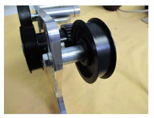
Fig. 6-c: Remove cog belt idler pulley
