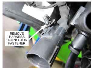
Fig. 9-e: Remove plastic harness connector fastener
