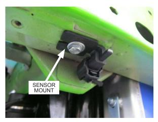
Fig. 7-ad: Reinstall ambient air temperature sensor as shown
