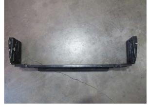
Fig. 4-e: Lower radiator support
