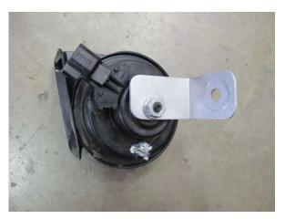
Fig. 7-j: New horn bracket
