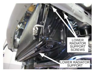
Fig. 2-w: Remove lower radiator support hardware
