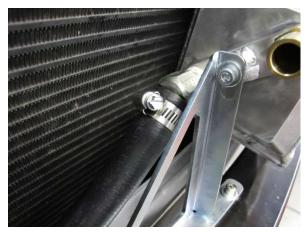
Fig. 9-k: Install long end of 150° molded hose to air/water cooler
