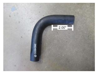
Fig. 8-e: Modify OEM breahter hose
