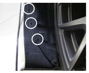
Fig. 2-c: Drill through and remove plastic rivets
