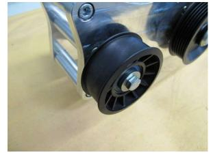
Fig. 6-b: Remove serpentine belt idler pulley
