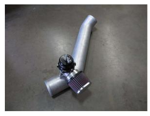
Fig. 7-aa: Install bypass valve to discharge tube 'B'
