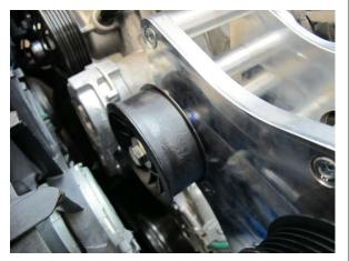
Fig. 6-h: Reinstall serpentine belt idler pulley
