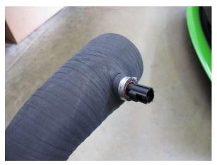
Fig. 7-y: Install IAT sensor to molded boss on discharge sleeve 'E'
