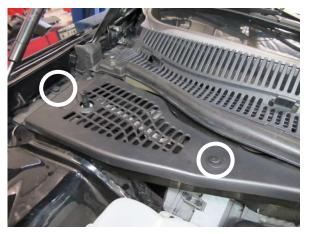
Fig. 1-d: Remove two plastic fasteners
