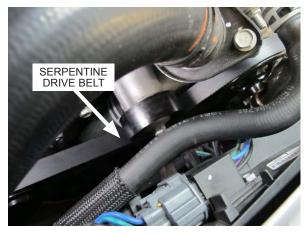
Fig. 6-i: Slide serpentine belt under OEM passenger side smooth idler pulley
