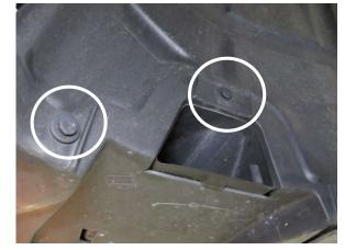
Fig. 2-d: Remove two plastic fasteners
