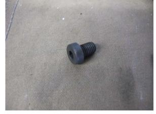
Fig. 9-h: Shorter front bumper support screw
