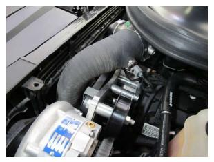
Fig. 7-z: Install discharge sleeve 'E' and reconnect IAT sensor
