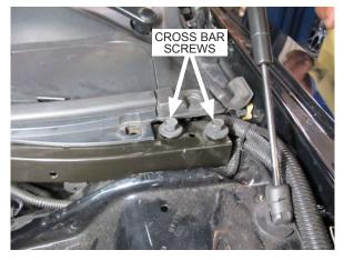
Fig. 1-c: Remove cross bar screws
