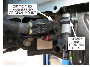
Fig. 9-f: Install the auxiliary water pump
