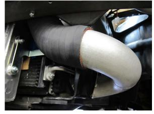
Fig. 7-w: Loosely install discharge tube 'D'
