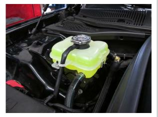
Fig. 9-z: Fill air/water cooling system with 50/50 water/coolant mix
