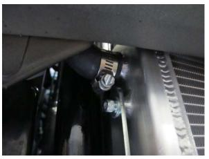
Fig. 9-j: Install short end of 150° molded hose to heat exchanger
