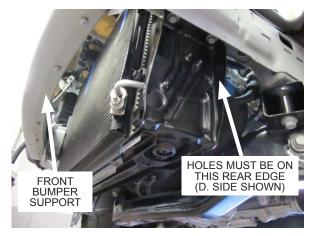
Fig. 4-k: Reinstall lower radiator support
