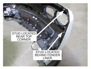
Fig. 2-h: Remove two nuts (Bumper removed for clarity)
