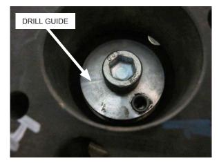
Fig. 3-b: Install drill guide
