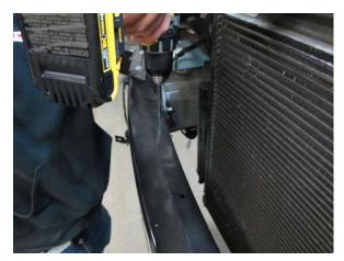
Fig. 7-n: Drill through two holes on front bumper support
