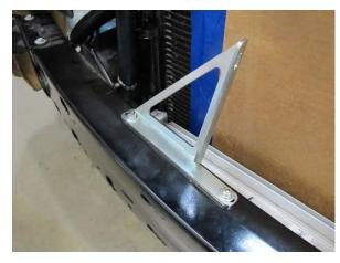
Fig. 7-o: Loosely install passenger side air/water cooler support bracket
