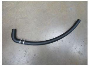
Fig. 5-e: Assemble new coolant reservoir hose as shown
