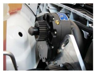
Fig. 8-c: Install supercharger to supercharger mounting bracket assembly
