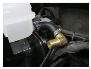
Fig. 9-q: Install hose and brass fitting assembly to air/water cooling system reservoir
