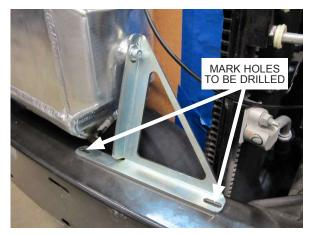
Fig. 7-r: Use driver side air/water cooler support bracket as drill template
