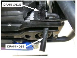
Fig. 2-s: Drain coolant
