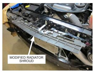
Fig. 10-f: Secure modified radiator shroud and three radiator shroud brackets
