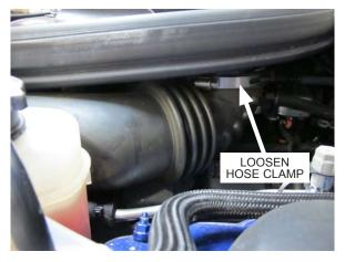
Fig. 2-o: Loosen hose clamp
