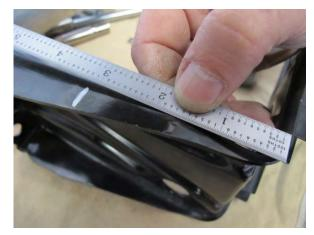
Fig. 4-f: Measure 3.25" from bottom edge
