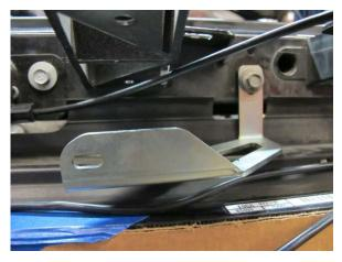
Fig. 7-I: Install upper air/water cooler support bracket
