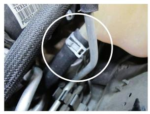
Fig. 5-g: Attach coolant hose to coolant reservoir
