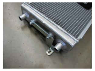
Fig. 7-e: Install passenger side heat exchanger bracket
