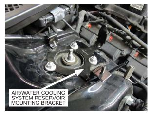
Fig. 9-I: Install air/water cooler system reservoir mount
