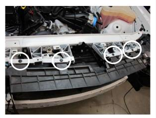
Fig. 2-m: Remove radiator shroud and fasteners
