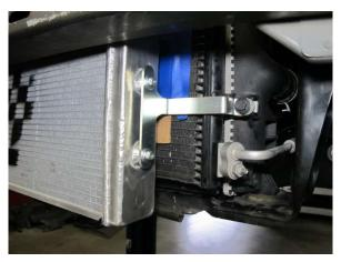
Fig. 7-h: Install driver side of heat exchanger assembly
