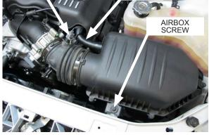
Fig. 2-q: Remove airbox and air inlet duct
