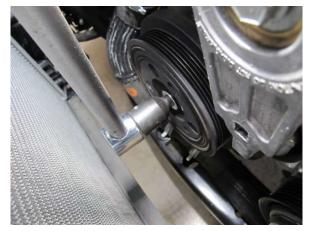
Fig. 3-a: Remove crankshaft damper bolt
