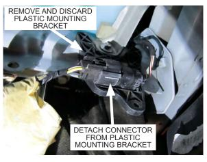
Fig. 2-i: Disconnect fog light connector
