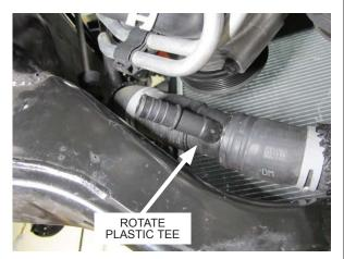
Fig. 5-d: Rotate plastic tee 180° clockwise
