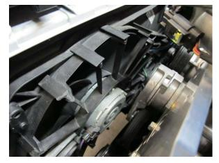
Fig. 4-c: Reinstall radiator fan assembly
