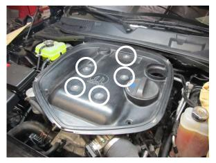
Fig. 2-p: Remove shaker base
