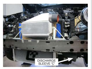
Fig. 7-v: Install air/water cooler
