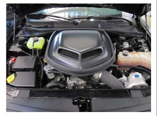
Fig. 11-f: Reinstall engine cover, shaker base, and shaker scoop
