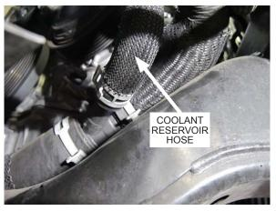
Fig. 5-b: Detach coolant reservoir hose from plastic tee
