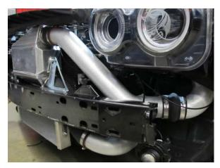
Fig. 8-i: Secure discharge tubes and discharge sleeves
