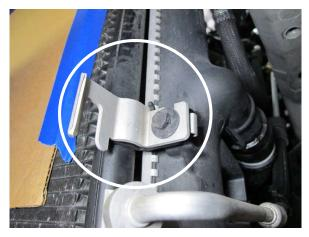
Fig. 7-c: Remove aluminum bracket and screw
