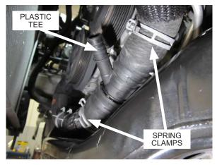
Fig. 5-c: Temporarily move two spring clamps
