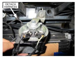
Fig. 7-i: Remove driver side horn
