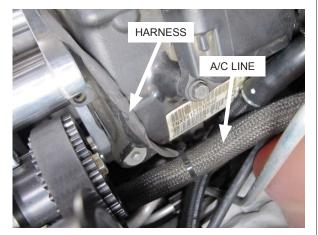
Fig. 6-k: Secure harness to A/C line
