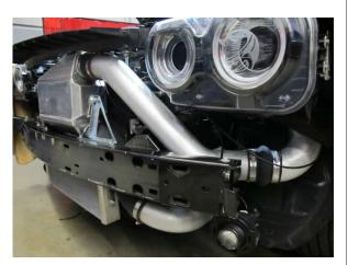
Fig. 7-ab: Install discharge tube 'B'
