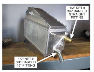
Fig. 7-a: Install fittings to air/water cooler
