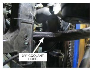
Fig. 9-t: Pass 3/4" coolant hose between radiator and core support
