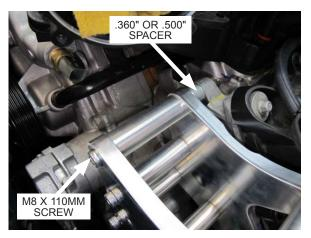
Fig. 6-f: Loosely attach S/C mounting bracket assembly to driver side cylinder head
