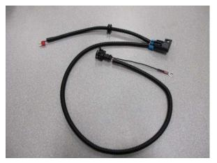
Fig. 9-a: Auxiliary water pump harness
