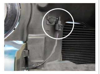
Fig. 2-I: Remove ambient air temperature sensor
