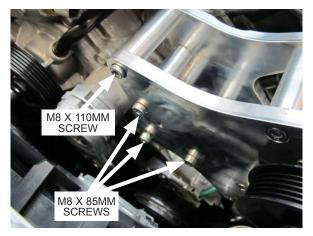
Fig. 6-g: Secure S/C mounting bracket hardware
