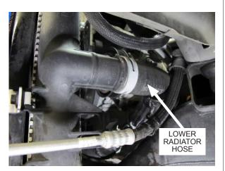
Fig. 4-d: Rettach lower radiator hose
