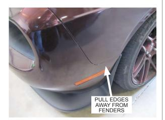
Fig. 2-j: Remove front bumper cover
