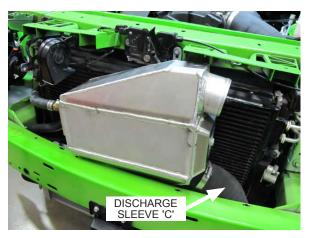
Fig. 6-u: Loosely install upper air/water cooler support bracket and air/water cooler
