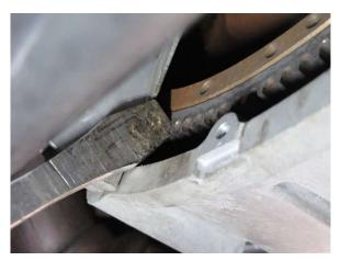
Fig. 3-g: Lock engine in position
