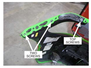
Fig. 2-h: Remove screws (Bumper removed for clarity)
