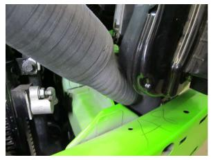
Fig. 6-ae: Adjust discharge sleeve 'B' and install driver side headlight
