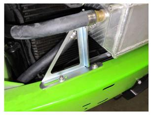
Fig. 6-w: Loosely install passenger side air/ water cooler support bracket
