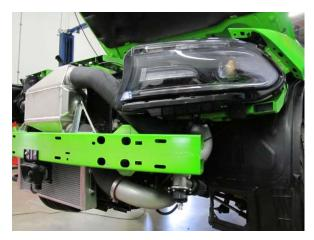
Fig. 7-i: Secure discharge tubes and discharge sleeves
