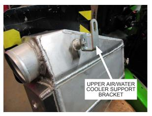
Fig. 6-n: Install upper air/water cooler support bracket
