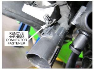
Fig. 8-e: Remove plastic harness connector fastener
