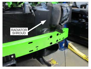
Fig. 2-k: Remove both radiator shrouds (Driver side shown)
