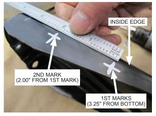
Fig. 4-e: Measure 2.00" up from first marks
