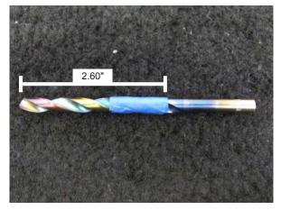
Fig. 3-c: Measure drill bit to 2.60"
