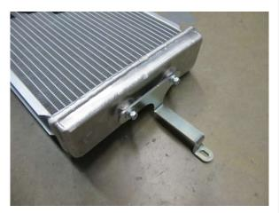
Fig. 6-g: Install driver side heat exchanger bracket
