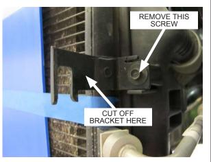
Fig. 6-d: Remove aluminum bracket and screw
