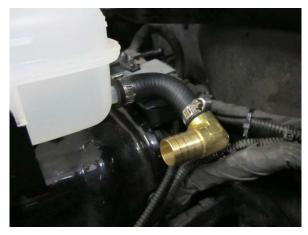
Fig. 8-q: Install hose and brass fitting assembly to air/water cooling system reservoir
