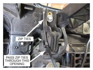
Fig. 2-o: Zip tie radiator to core support
