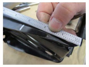
Fig. 4-c: Measure 3.25" from bottom edge
