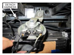
Fig. 6-j: Remove driver side horn
