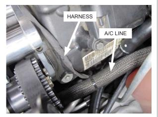
Fig. 5-k: Secure harness to A/C line
