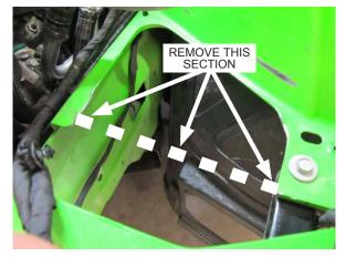
Fig. 6-b: Modify driver side inner wheel well as shown
