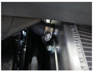
Fig. 8-j: Install short end of 150° molded hose to heat exchanger
