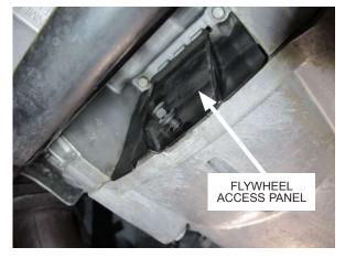
Fig. 3-f: Remove transmission access panel
