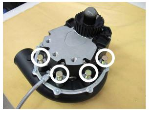
Fig. 7-b: Lubricate supercharger mounting boss threads
