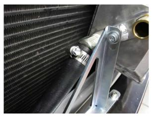
Fig. 8-k: Install long end of 150° molded hose to air/water cooler
