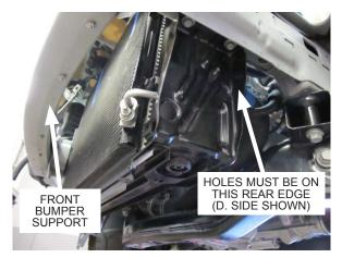
Fig. 4-h: Reinstall lower radiator support
