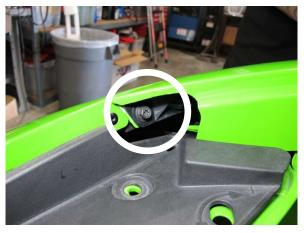
Fig. 2-g: Remove each upper front bumper cover screw
