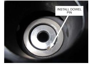
Fig. 3-e: Install dowel pin
