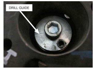
Fig. 3-b: Install drill guide
