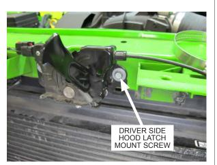
Fig. 6-m: Remove driver side hood latch mount screw
