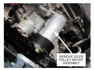
Fig. 2-s: Remove idler pulley mount assembly
