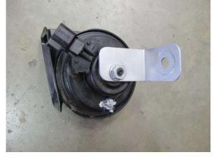
Fig. 6-k: New horn bracket
