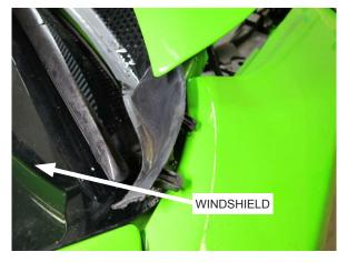
Fig. 1-c: Detach windshield cowl from passenger side fender
