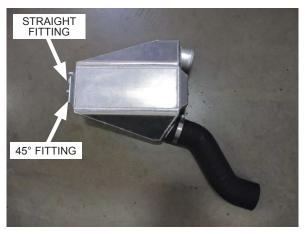
Fig. 6-t: Install discharge sleeve 'C' to the air/water cooler as shown
