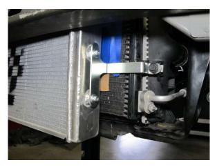
Fig. 6-i: Install driver side of heat exchanger assembly
