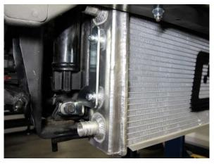
Fig. 6-h: Install passenger side of heat exchanger assembly
