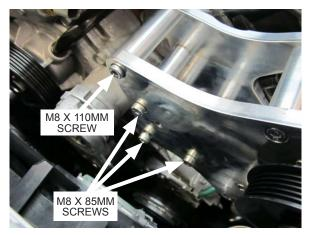
Fig. 5-g: Secure S/C mounting bracket hardware
