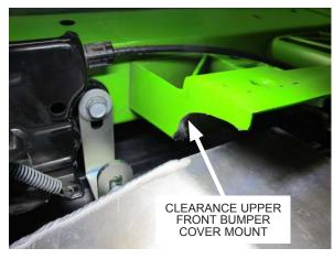
Fig. 6-o: Clearance the front bumper cover mount
