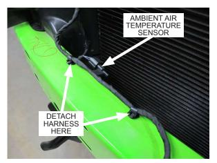
Fig. 2-j: Detach adaptive cruise control harness
