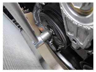
Fig. 3-a: Remove crankshaft damper bolt
