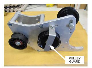
Fig. 5-a: Remove pulley guard
