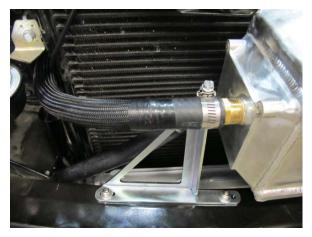
Fig. 8-u: Attach 3/4" coolant hose to air/water cooler
