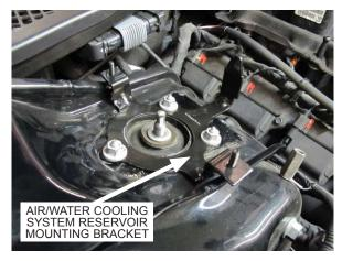
Fig. 8-I: Install air/water cooler system reservoir mount
