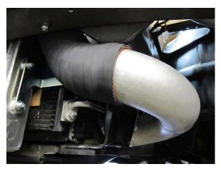
Fig. 6-y: Loosely install discharge tube 'D'
