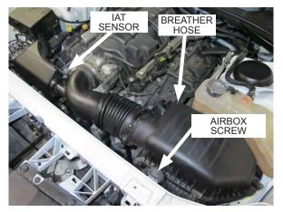
Fig. 2-m: Remove airbox and air inlet duct
