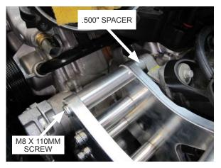
Fig. 5-f: Loosely attach S/C mounting bracket assembly to driver side cylinder head
