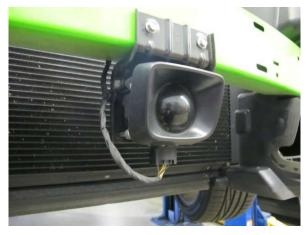
Fig. 2-i: Disconnect adaptive cruise control sensor
