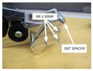
Fig. 5-d: S/C mounting bracket hardware
