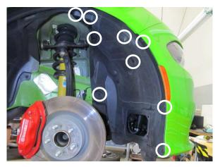
Fig. 2-c: Remove fender liner fasteners
