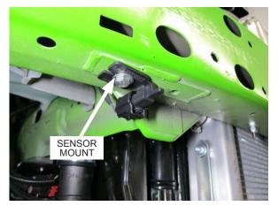
Fig. 6-ah: Reinstall ambient air temperature sensor as shown
