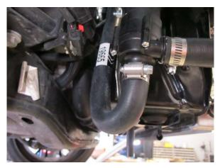
Fig. 8-x: Install coolant hose to electric water pump inlet
