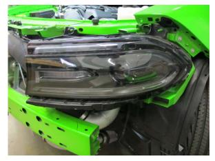
Fig. 6-ac: Remove driver side headlight
