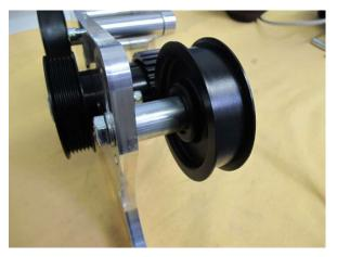
Fig. 5-c: Remove cog belt idler pulley
