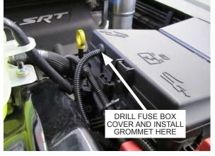
Fig. 8-b: Drill fuse box cover, install grommet and route wire into fuse box
