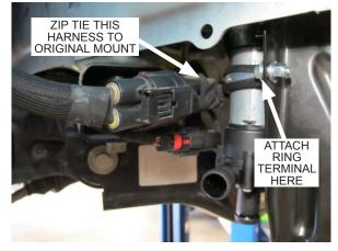
Fig. 8-f: Install the auxiliary water pump
