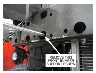
Fig. 8-g: Remove front bumper support screw
