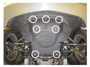
Fig. 2-d: Remove engine service panel fasteners
