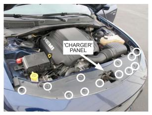
Fig. 2-a: Remove upper front bumper fasteners
