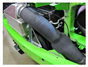
Fig. 6-ad: Install discharge sleeve 'B'
