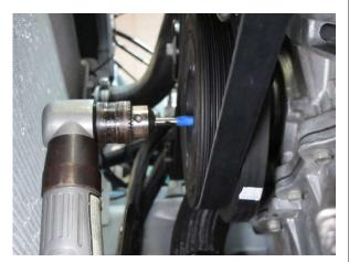
Fig. 3-d: Drill crankshaft / damper assembly
