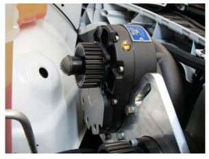
Fig. 7-c: Install supercharger to supercharger mounting bracket assembly
