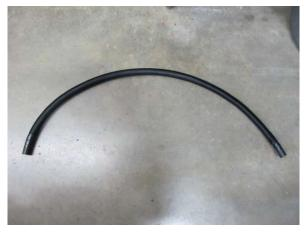
Fig. 8-n: 44" length of the 3/4" coolant hose
