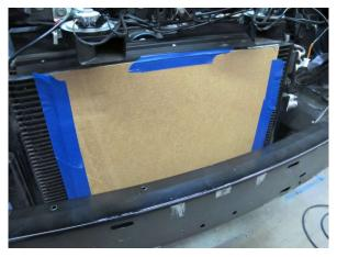
Fig. 6-c: Cover A/C condenser with cardboard
