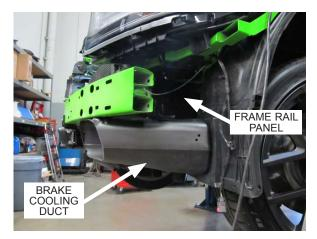
Fig. 2-I: Remove both brake cooling ducts (Driver side shown)
