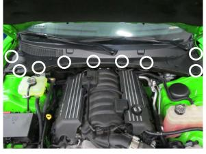
Fig. 1-b: Remove plastic fasteners
