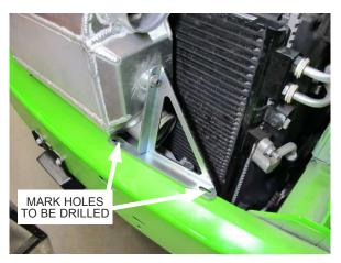
Fig. 6-q: Mark the two holes to be drilled on the driver side of the front bumper support
