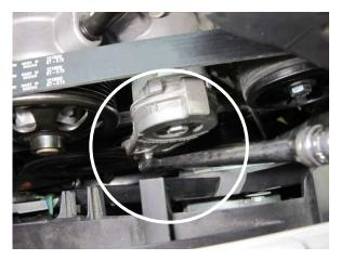
Fig. 2-r: Remove accessory drive belt
