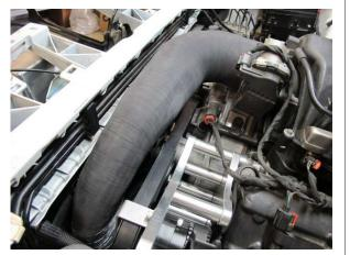
Fig. 6-ab: Install discharge sleeve 'E' and reconnect IAT sensor
