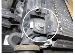
Fig. 6-e: Remove screw
