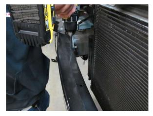
Fig. 6-r: Drill holes in front bumper support
