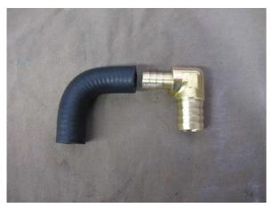
Fig. 8-p: Insert brass fitting to 1/2" x 90° coolant hose elbow
