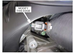
Fig. 9-b: Modify driver side engine cover
