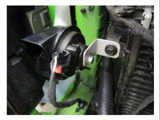
Fig. 6-I: Relocate driver side horn to upper radiator
