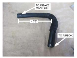
Fig. 7-e: Modify OEM breahter hose
