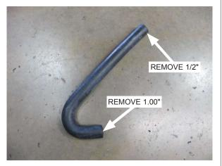
Fig. 8-i: Modify 150° molded hose as shown
