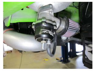
Fig. 7-k: Attach vacuum hose to bypass valve
