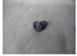
Fig. 8-h: Shorter front bumper support screw
