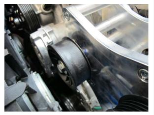
Fig. 5-h: Reinstall serpentine belt idler pulley
