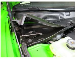
Fig. 1-d: Lift up passenger side of winshield cowl
