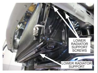
Fig. 2-p: Remove lower radiator support hardware
