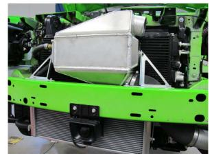
Fig. 6-x: Install air/water cooler
