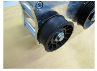
Fig. 5-b: Remove serpentine belt idler pulley
