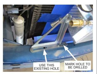
Fig. 6-p: Mark the holes to be drilled on the passenger side of the front bumper support
