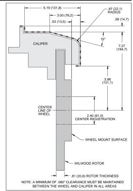
Figure 2. Wheel Clearance Diagram
