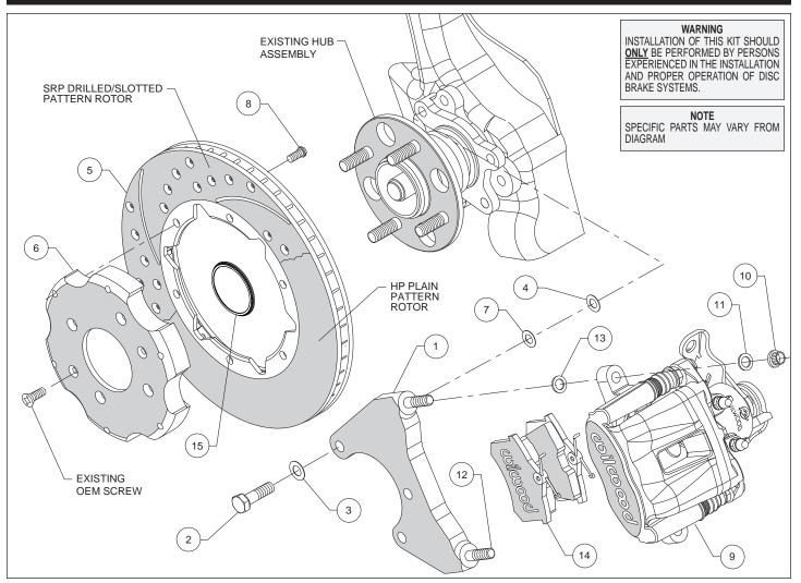
Figure 1. Typical Installation Configuration
