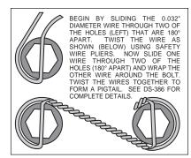
Figure 3. Safety Wire Diagram
