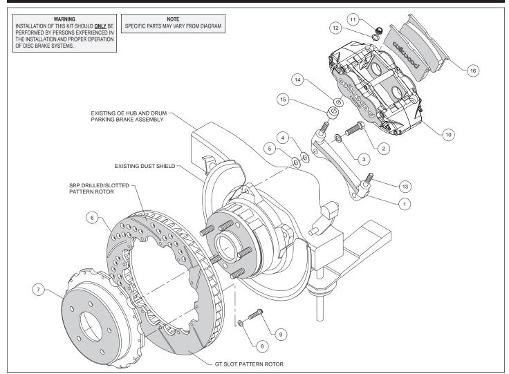
Figure 1. Typical Installation Configuration
