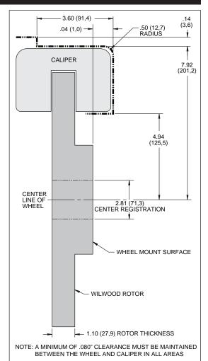
Figure 2. Wheel Clearance Diagram
