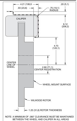
Figure 2. Wheel Clearance Diagram
