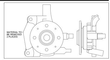
Figure 3. Spindle Modifications
