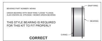
Figure 2. Loose Fit Bearing Configuration
