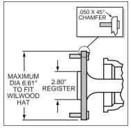
Figure 5. Axle Flange Maximum Dimension
