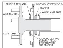
Figure 6. Retainer / Axle Diagram
