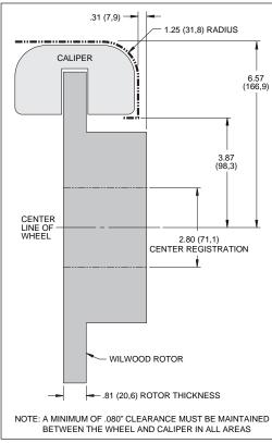
Figure 4. Wheel Clearance Diagram
