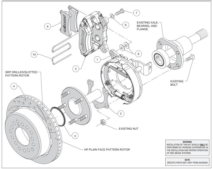
Figure 3. Typical Installation Configuration
