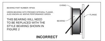
Figure 1. Press Fit Bearing Configuration
