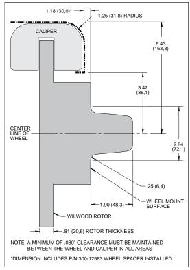
Figure 2. Wheel Clearance Diagram
