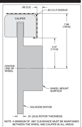
Figure 2. Wheel Clearance Diagram
