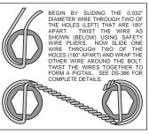
Figure 3. Safety Wire Diagram
