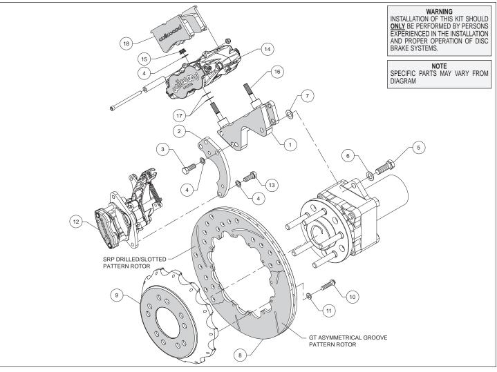
Figure 1. Typical Installation Configuration Page 2
