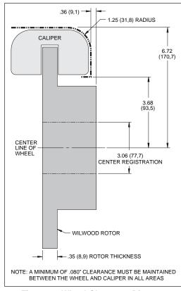
Figure 2. Wheel Clearance Diagram
