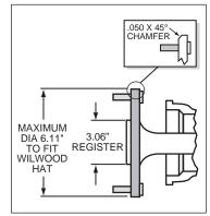
Figure 3. Axle Flange Maximum Dimension
