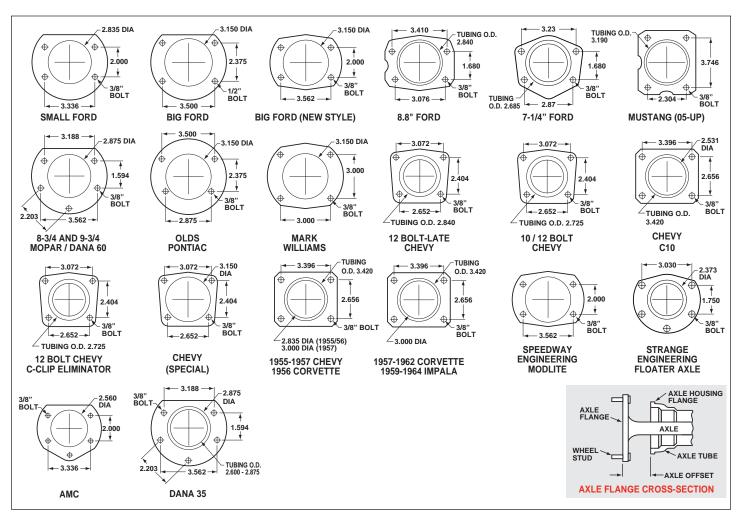
Figure 6. Rear Housing Flange Chart and Axle Flange / Cross-Section
