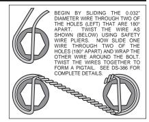
Figure 4. Safety Wire Diagram
