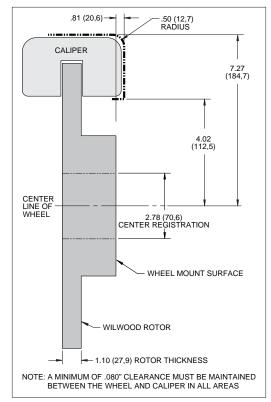
Figure 3. Wheel Clearance Diagram
