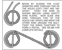
Figure 4. Safety Wire Diagram
