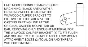
Figure 3. Machining Diagram
