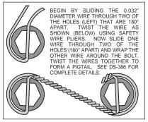
Figure 4. Safety Wire Diagram
