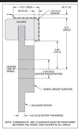
Figure 2. Wheel Clearance Diagram
