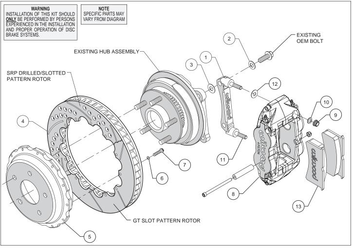
Figure 1. Typical Installation Configuration
