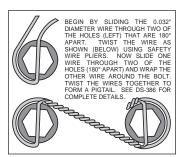
Figure 4. Safety Wire Diagram
