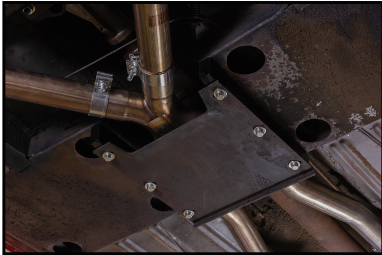
SHOWN ABOVE BRACE SPACER KIT INSTALLED
