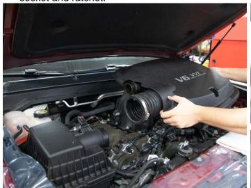
7. Carefully lift the engine cover along with the factory airduct and place it aside.
