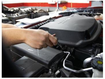
5. Loosen the throttle body clamp using an 8mm socket and ratchet.
