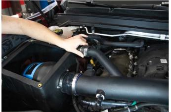
11. Insert the factory hose into the duct as shown.
