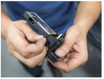
12. Remove the factory MAF sensor gasket shown above and place it aside. Keep the MAF sensor for use with the Volant Air Intake.
