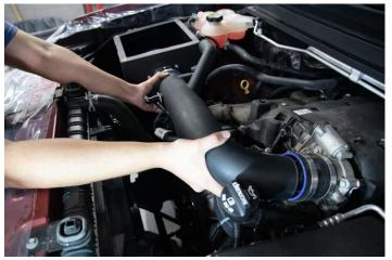
10. Insert the duct into the straight sleeve on the throttle body and the hump hose on the airbox as shown.
