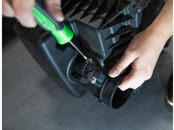
11.Remove the 2 Torx screws holding the factory MAF sensor using a T-20 Torx screwdriver.
