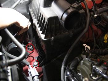
8. Using a 10mm socket and a ratchet with extension, remove the 2 nuts shown above. Keep 1 nut for use with installing your Volant Intake
