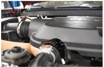
4. Unclip the vent line fitting by pressing on the side and pulling it gently.
