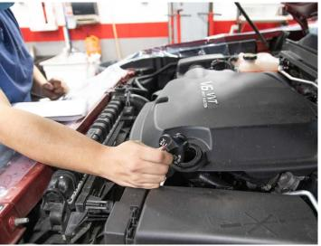
6. Remove the engine oil cap.
