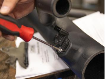
2. Use the two Philips head screws and screw the MAF sensor to the duct securely.
