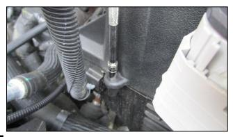
**4.** Install Volant air box onto lower portion of factory air box in vehicle. Using the three factory screws from removal step 7, secure Volant air box with a ratchet and 8mm socket with extension.
