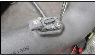
Install sensor into Volant air duct. Secure using the two supplied screws and a Philips head screwdriver.
