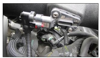
**11.** Re-route MAF wiring harness under large wiring harness and install into MAF sensor until it clicks into place. Push red tab back down to lock sensor in place.
