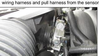
**3.** Loosen clamp securing factory air duct to throttle body with a ratchet and 8mm socket.
