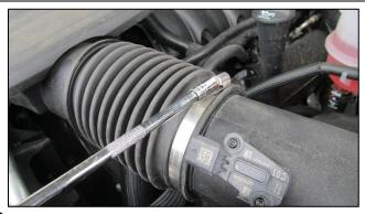
Loosen clamp securing factory air duct to the factory air box with a ratchet and 8mm socket.
