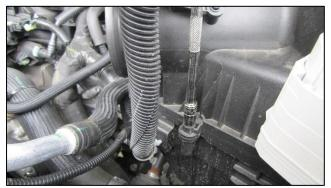
**1.** Remove three bolts securing factory air box upper portion to lower using a ratchet with extension and 8mm socket.
