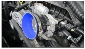
**6.** Place reducer onto throttle body with included #56 clamp on smaller diameter. Place included #64 clamp on larger diameter.
