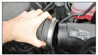
**5.** Pull air duct bellows from air box. Remove air duct from throttle body.
