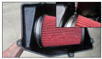
**3.** Install filter onto adapter in Volant air box. Tighten clamp using a ratchet and 8mm socket.
