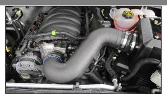
**1.** Insert Volant air duct into hump hose and reducer.
