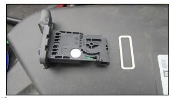
**12.** Remove factory gasket from MAF sensor.
