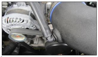
**10.** Push other end of breather hose onto installed elbow fitting in Volant air duct.
