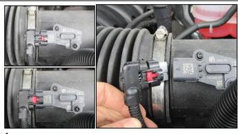
Pull red tab on MAF sensor wiring harness.
