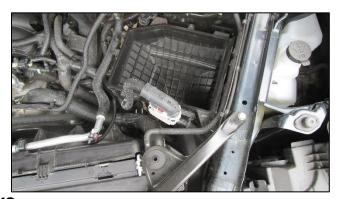
**10.** Lower factory air box remains in vehicle and is used with Volant air intake.
