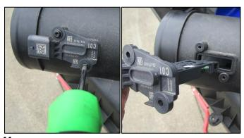
**11.** Remove two screws securing MAF sensor with a T20 Torx driver. Remove MAF sensor from factory air box.
