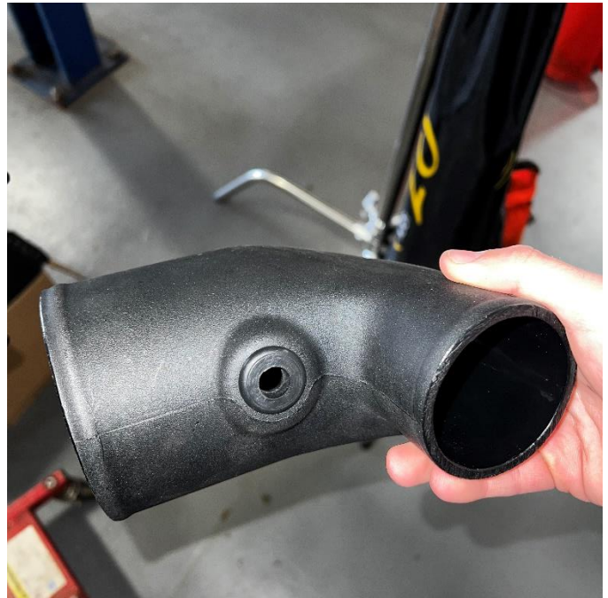
2. Install the rubber grommet into the Volant air duct.
