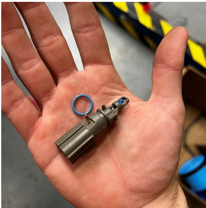
3. Remove the O-ring from the temperature sensor.
