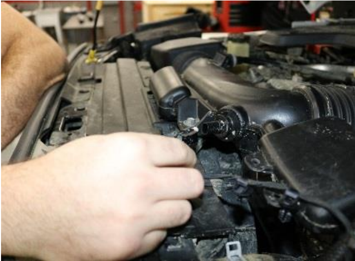
1. Unclip wiring harness from air temp sensor.
