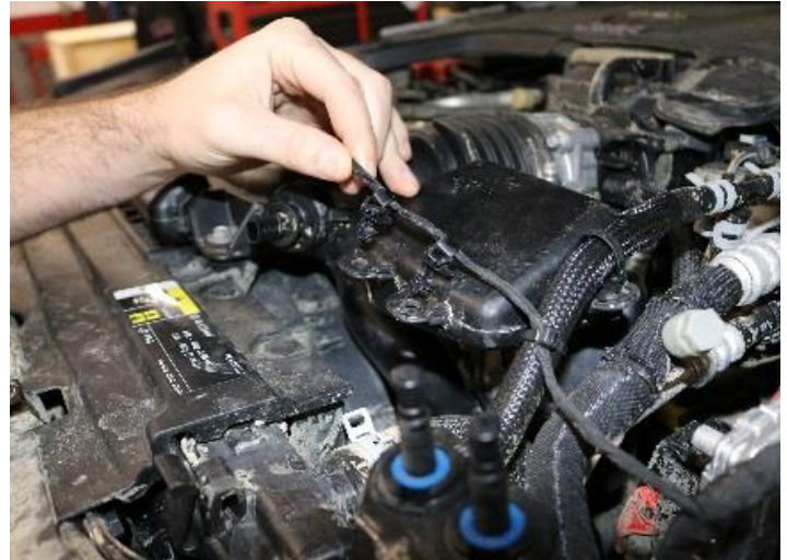
2. Using trim removal tool, remove the (2) clips attaching the ATS wiring harness to the factory air duct.
