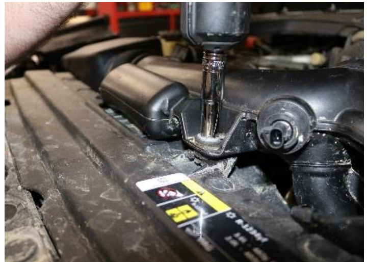
4. Remove the two 10mm bolts holding the factory air duct to the core support using a 10mm socket and ratchet.
