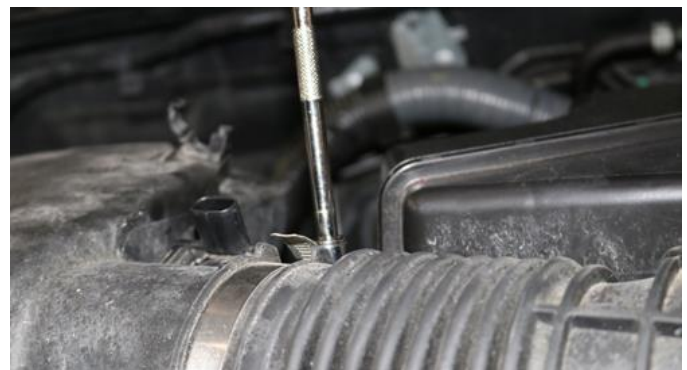
5. Loosen two clamps from the factory air duct using ratchet and 10mm socket.
