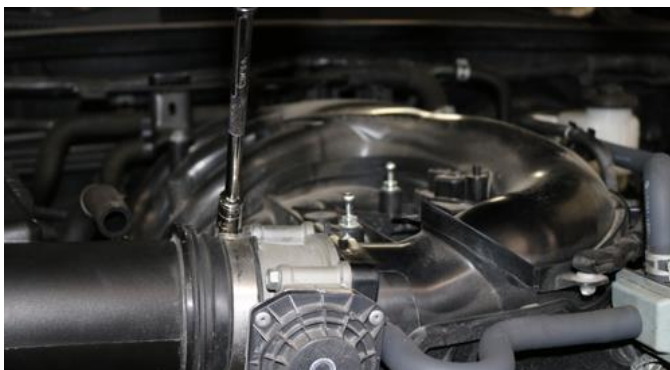
5. Loosen two clamps from the factory air duct using ratchet and 10mm socket.
