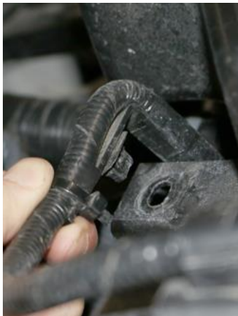
3. Undo two MAF sensor wire retaining clips.
