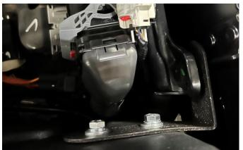
7. Insert push clip on factory wiring harness mount into hole on bracket
