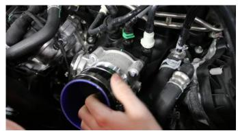
10.Install two #56 clamps onto the straight sleeve and place the straight sleeve on the throttle body.
