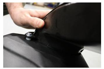
3. Attach the factory air scoop onto the Volant air box using a 10mm and socket and wrench. Using the provided hardware; place the .625" flat washer on the M6-25mm bolt through the factory mounting location of scoop. Place the provided .25" spacer between the scoop and Volant air box. On the inside of the air box place the .75" flat washer on bolt, followed by lock washer and M6 nut.
