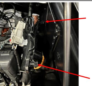
11.Using a trim removal tool, carefully pull the plastic wiring harness mount from the inner fender.
