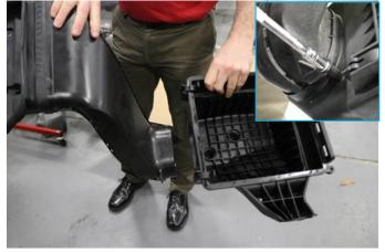
10. Remove the bolt holding the factory air scoop to the air box using an 8mm socket. Separate the scoop from box and save it for Install Step 3.
