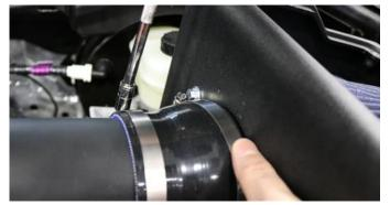
12. Insert the air duct onto the straight sleeve on the throttle body and large end of reducer onto the filter adapter. Adjust Volant air duct to proper fit and tighten all clamps using an 8mm socket or flat head screwdriver. **NOTE:** Also tighten the filter's clamp at this time.
