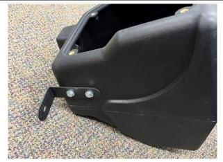
1. Install wiring harness bracket to Volant air box using two 6mm x 16 bolts, two .25" x .63" flat washers, two .25" lock washers and two 6mm nuts.
