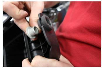
9. Remove the metal bushing and rubber grommet from the factory air scoop. Save metal bushing and rubber grommet for **Install Step 2**.
