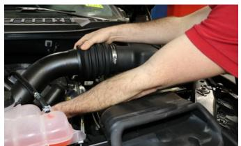
4. Unclip the air box lid and remove the factory duct and lid assembly as one piece.
