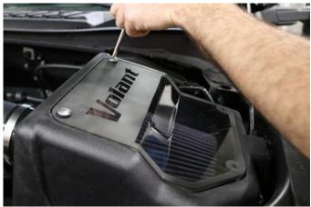
14.Install the Volant lid using the provided 4 truss head screws with rubber washers and Philips head screwdriver.
