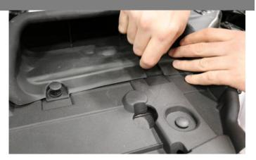
6. Re-install the factory scoop with clips saved from **Removal Step 8**.
