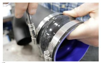
**13.** Install the hump hose onto the Volant air duct along with two #64 clamps and tighten using a ratchet and 8mm socket or flat head screwdriver. Leave clamp on open end of hump hose loose.
