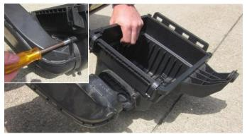
**8.** Remove the bolt attaching the scoop to factory air box using an 8mm socket. Remove the factory air scoop from the bottom of the air box.
