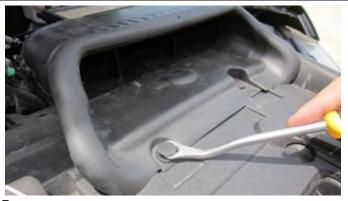
**6.** Remove the two plastic clips from the factory air scoop. Save clips for Install Step 8.
