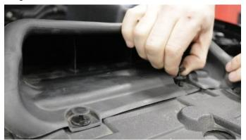
**B.** Reinstall factory scoop and attach with clips from **Removal Step 6**.
