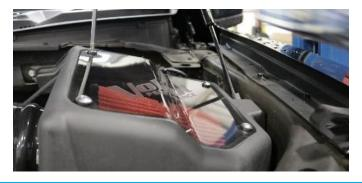
**19.** Install lid using provided 4 truss head screws with rubber washers and Philips head screwdriver.
