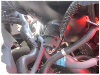
1. Disconnect the harness from the air temperature sensor on back side of factory air duct.
