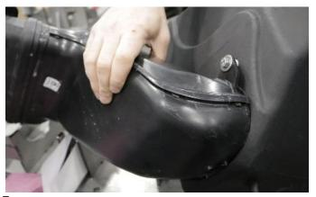
**5.** Install factory scoop to Volant air box using provided 6mm-25 bolt with flat washers, lock washer, spacer, and nut using 10mm socket or wrench.
