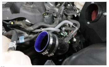
**14.** Install the straight sleeve onto lower factory inlet with #64 clamp. Tighten clamp using a ratchet and 8mm socket or flat head screwdriver. Leave clamp on open end of straight sleeve loose.
