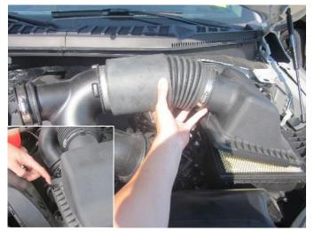
**3.** Unclip the air box lid and remove the factory duct and lid assembly as one piece.
