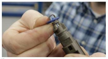
**II.** Remove O-ring from the temp sensor.
