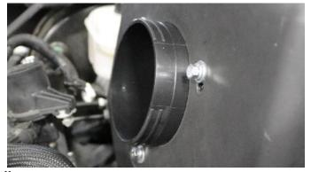
**11.** Attach the filter adapter to the Volant air box using the provided 3 bolts, flat washers, and lock washers and a 10MM wrench or socket.
