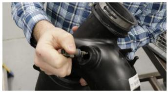
**9.** Remove the air temp sensor from factory duct. Save for **Install Step 12**.
