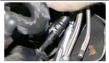
**1.** Unclip the quick disconnect vent hose.
