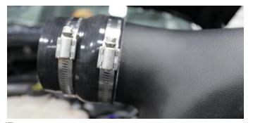
15. Insert larger end of reducer onto Volant air duct using #56 clamp. Place #48 clamp on the smaller side. Tighten #56 clamp only using a ratchet and 8mm socket or flat head screwdriver.
