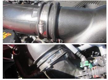
2. Loosen the clamps on the top and bottom intake tubes using a ratchet and 7mm socket or flathead screwdriver.
