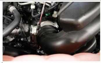
Loosen the throttle body clamp using a 7mm socket.
