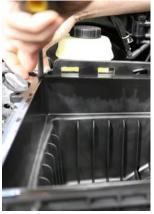
**6.** Use a pry tool to remove the three wire retention clips.
