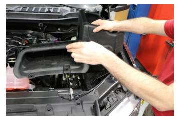
**3.** Install the factory air scoop, and Volant air box into vehicle making sure to place the studs on the bottom of the air box into factory grommets.
