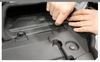
**5.** Re-install the factory scoop with clips saved from Removal Step 8.
