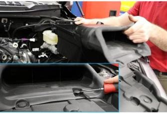
**8.** Remove the two clips holding the factory scoop using a pry tool. Save clips for **Install Step 5**. Remove scoop and air box assembly from vehicle.
