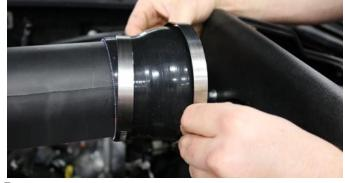
Install one #56 clamp on small end of the reducer, and one #64 clamp on larger end of reducer. Place small end of reducer onto straight end of Volant air duct.
