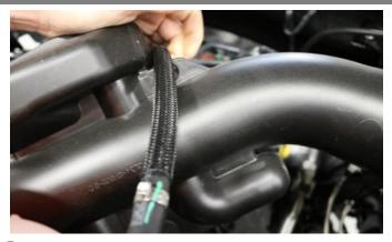
Release the coolant hose from the factory air duct
