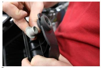
**9.** Remove the metal bushing and rubber grommet from the factory air scoop. Save metal bushing and rubber grommet for **Install Step 1**.
