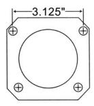
This kit is for axles with a 3 1/8" spread center to center on the top two bolt holes (pictured left). If your axle flange does not measure this, please Call 800.405.2000 for further assistance.
