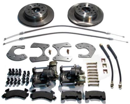
This kit is for Ford 9" rear axles with the small (2.835") style bearing and Ford 8" rear ends. This kit is designed to work with axles with either GM 5 x 4.75 Bolt Pattern and 7/16" wheel studs or Ford 5 x 4.5 Bolt Pattern and 1/2" wheel studs. Rotor center measures 2.78".
