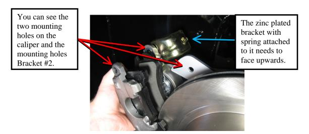
With the caliper on the rotor and in Bracket #2 we can use the two caliper bolts to secure the caliper in place using a 3/8" allen wrench and torque to factory specs.
