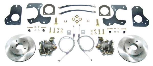
This kit is for GM G Body & some S-10, S-15, F Body's 1978 - 2004. The axle flange has three holes. The bottom two holes measure 2 11/16" center to center, and the top hole is 5 3/8" above those two holes. This kit is designed to work with axles with either GM 5 x 4.75 Bolt Pattern and 1/2" wheel studs.
