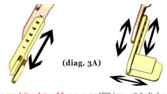
Upon completion of steps 1-3, once you are 100% happy with the fit of your restraint, we recommend that at this time your remove all screws one at a time (except screw #2 in step 2) and secure them with tread lock "blue" and tighten snug.
