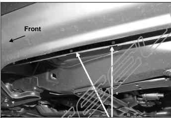
(Fig 1) Driver side front mounting location pictured
