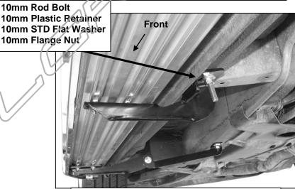
(Fig 11B) Driver side Center Bracket pictured
