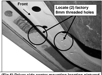
(Fig 6) Driver side center mounting location pictured
