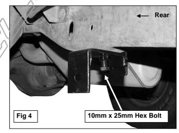
Loosen 10mm Locking Bolt in Frame Bracket to slide Bracket Assembly forward or backward on frame channel to line up with the end of the Sidebar. Once properly lined up, tighten 10mm Lock Bolt
