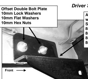
(Fig 3) Front Mounting Bracket installation
