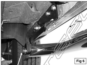
Secure the Sidebar to the Mounting Brackets with: 1/2" x 2" Hex Bolts 1/2" Flat Washers 1/2" Lock Washers
