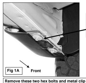
nuts. Drill a 3/8" hole through the pinch weld to clearance holes ONLY if necessary
