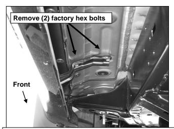
(Fig 1) Driver/Left Front Mounting Location Pictured
