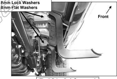
(Fig 4) Driver/Left Center and Rear Brackets Pictured
