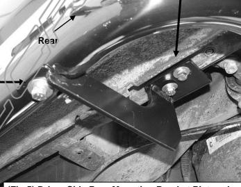
(Fig 5) Driver Side Rear Mounting Bracket Pictured
